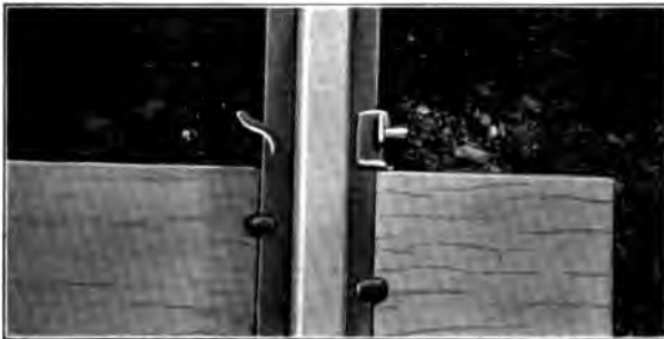
2. Showing Vaughan Rail Anchor after application to rail. Note that it does not have its final grip on the rail in this position. Spring should be driven to diagonal position shown in cut to the right.
